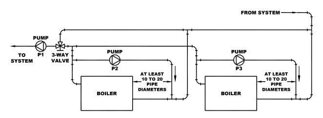
Figure 2 By-Pass Piping Using Three-Way Valve – Multiple Boilers
